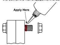
1. For Blind Holes, apply several drops down the female threads into the bottom of the hole. As threads are engaged, compressed air forces the product upwards into the threads.
