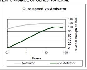
(After 24 hr at 22  $^{\circ}$ C on degreased 3/8-16 steel Grade 8 nuts and Grade 5 bolts)
